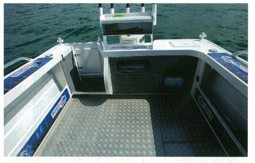
Conversely, the Trident's cabin sides go virtually out to the sides so crew are not encouraged to walk around the sides, but instead use the fore-hatch for anchor work.
