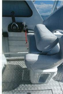
well above the ordinary tinnie. You also get good gear like hydraulic steering, flush-mount throttle and curved Perspex windscreen without 'blind spots.' Our test boat didn't seem to have footrest fitted, but they are included in the specifications!
